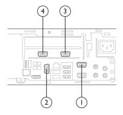
**1 and 2:** Powered Configurable serial port expansion card installation that supplies two additional serial ports (COM3 and COM4) **3 and 4:** Two Power Configurable serial ports, COM1 and COM 2, are standard on the POS System.
